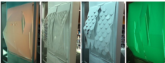
Figure 5. Four different corrugated panel designs, actuated.
